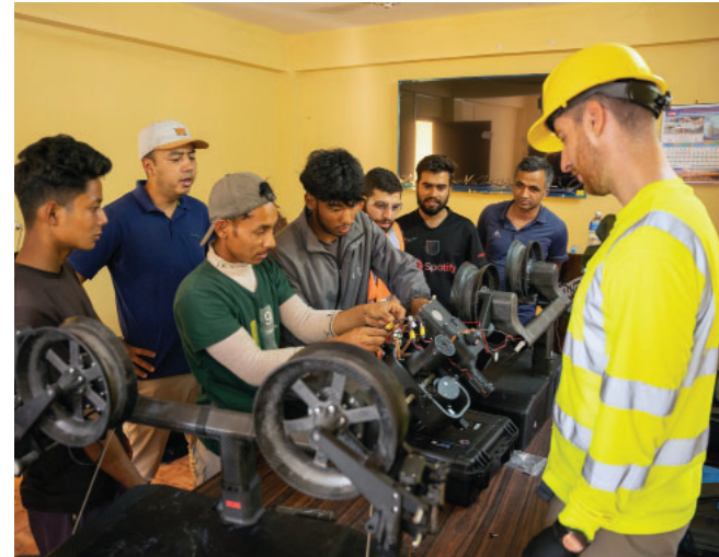
Technology and knowledge transfer to retrofit transmission lines using a remote controlled robot applying photonic coating
